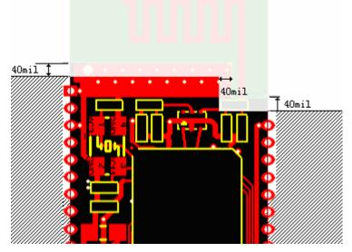
As you see above, trying to remove metal under antenna is good for RF radiate.
