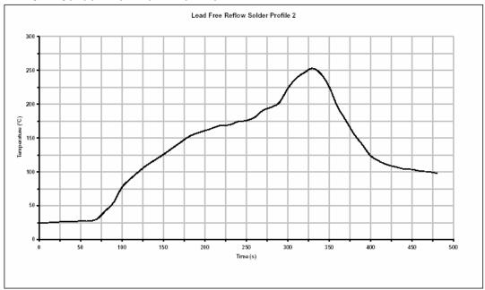
Typical Lead-Free Re-flow Solder Profile
